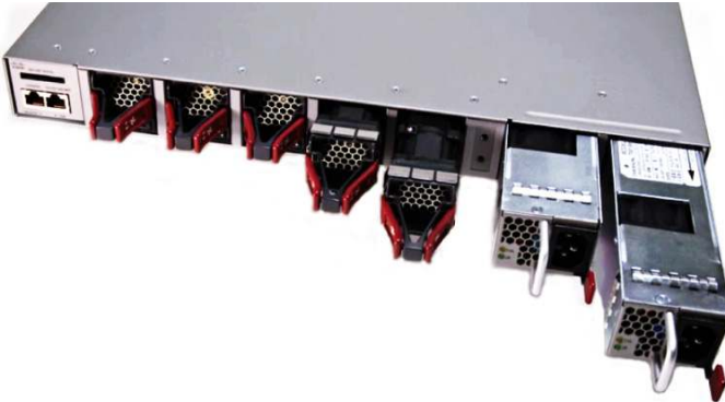
Figure 7. Redundant Fan and Power Supply
